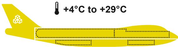
**4** independently controlled temperature zones offering the right thermal environment for temperature-sensitive dangerous goods
